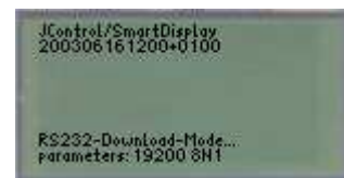
Fig. 4: Splash screen of the system download mode
